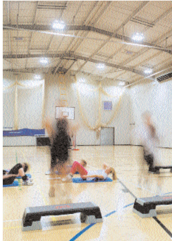
An area elastic beech floor, walls of the right reflectance value and compact fluorescent lights between badminton courts provide an excellent sports hall environment.
