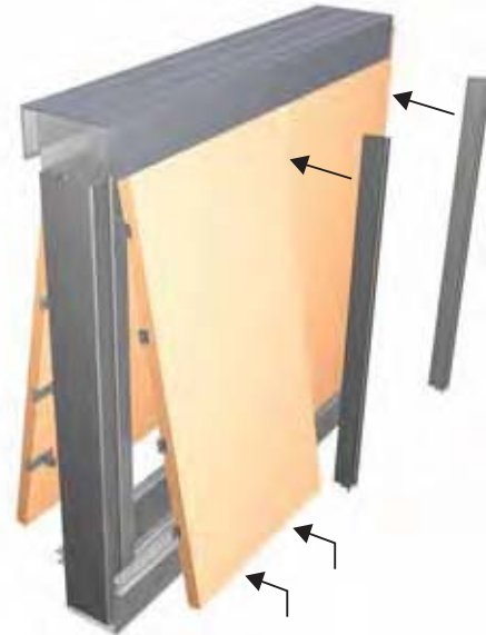
Tenon Bi-element construction with push fit trim sections
