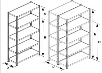
Height to depth ratio -Single-Sided Bays/Runs Height to depth ratio -Double-Sided Bays/Runs D = depth
