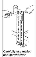
and screwdriver blade to tap down the plate to ensure it is fully located.
