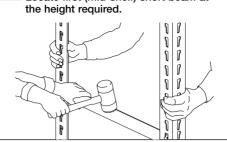
Locate top short beam, position at highest shelf position required. 1 1 1
