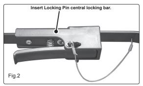
3.7 To remove the carrier, remove the safety locking pin and squeeze the lever on the central locking bar while pulling the locking bar upwards. The locking bar will now fold upwards releasing the carrier from the tow ball.
